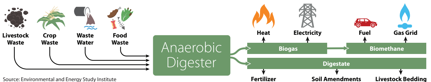
Figure 1: Anaerobic Digestion Process
